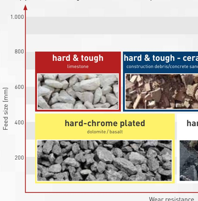
This illustration helps you to choose the optimum impact bars for normal crushing operations.
